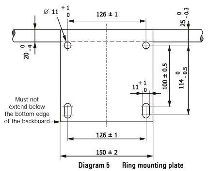
For existing basket support structures, it is recommended that the ring mounting plate be fixed to the framework according to the measurements given in Diagram 6.
