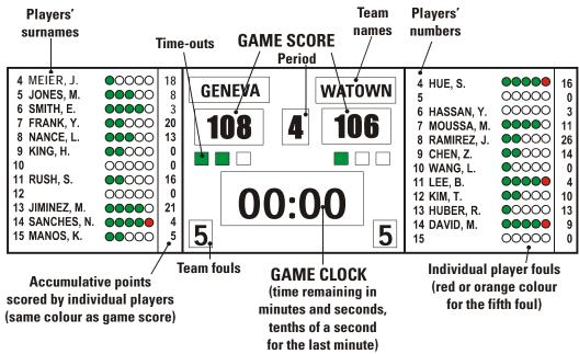
Diagram 8 Scoreboard for Level 1 (example of the layout)
