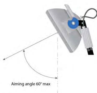
Forbidden area for lighting mountings to avoid glare towards the main camera
