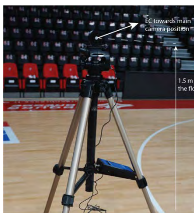
Main camera illuminance (EC) measurement
