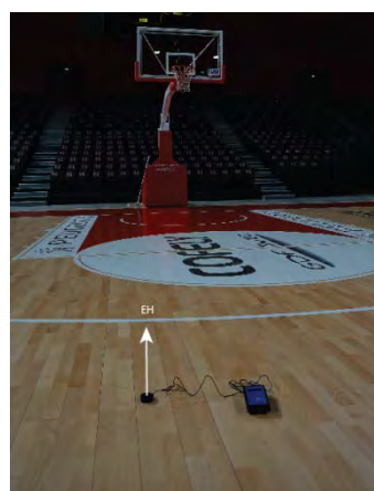
Horizontal illuminance (EH) measurement
